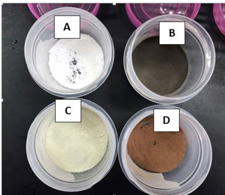
Figure 1: Photocatalyst powder (A) blank \text{TiO}_2 , (B) Fe- \text{TiO}_2 , (C) Cu- \text{TiO}_2 and (D) Co- \text{TiO}_2
