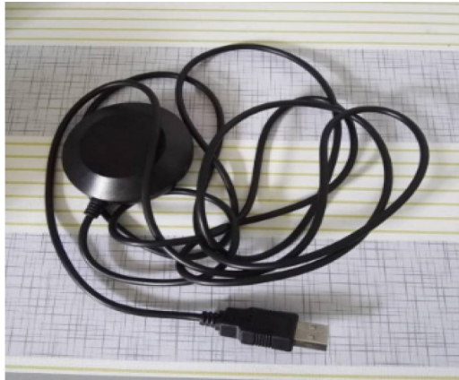
Figure 1: Antenna of the GPS system used to collect data transmitted by satellites.
