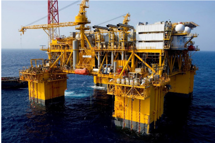
Figure 1: Typical deep-draft semi-submersible
