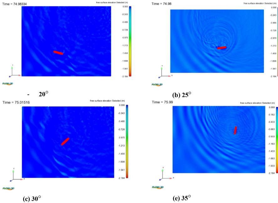
Figure 7: Free surface elevation of complete turning circle at rudder's angle (a) 20°, (b) 25°, (c) 30° and (d) 35°
