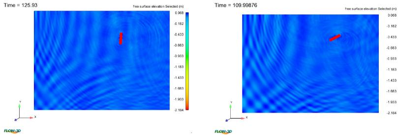
Figure 9: Free surface elevation of complete turning circle at 8 knots (left) and 9 knots (right)
