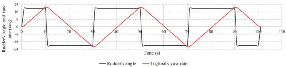
Figure 4: Zig zag graph of tugboat manoeuvre at rudder's angle  $20^\circ/20^\circ$
