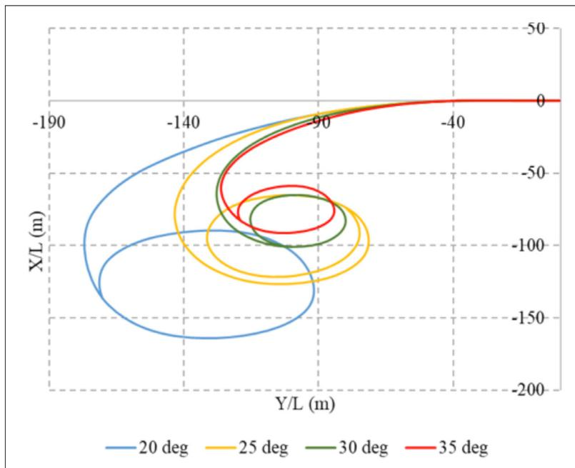
Figure 5: Graph of turning diameter at various rudder’s angles
