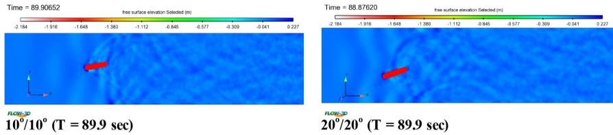
Figure 5: Free surface elevation of zig zag manoeuvre for 10°/10° (left) and 20°/20° (right) rudder’s angle
