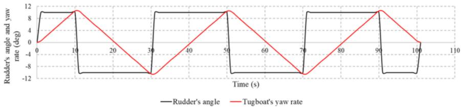
Figure 3: Zig zag graph of tugboat manoeuvre at rudder's angle  $10^\circ/10^\circ$
