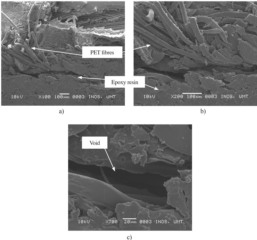
Figure 6: SEM micrograph of the cross section of 10 wt% PET/epoxy (PTE) composites at a) 100× magnification b) 200× magnification and b) 700× magnification
