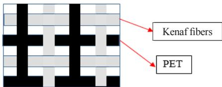
Figure 1: The interwoven fabric containing kenaf and PET fibres
