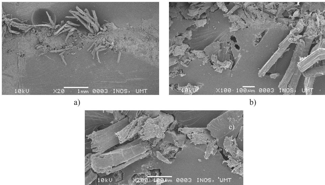
Figure 8: Micrographs of the cross section of 8% kenaf/PET/epoxy (KPTE) composites at a) 20× magnification b) 100× magnification and c) 200 × magnification
