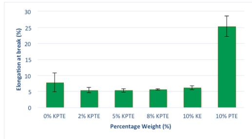
Figure 4: Elongation at break of epoxy and its composites.
