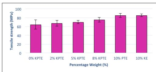
Figure 2: Tensile strength of epoxy and epoxy-based composites
