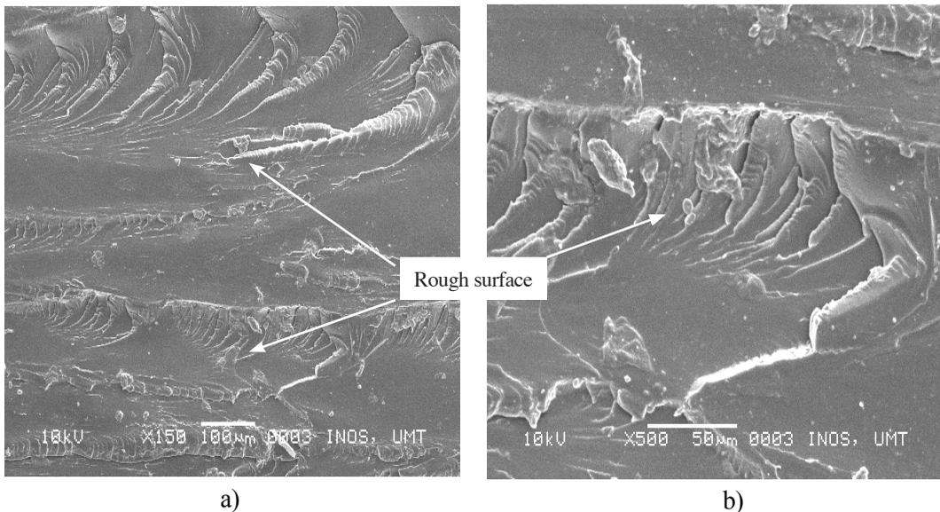
Figure 5: SEM micrograph of the cross section of pure resin under a) 150 × magnification and b) 500× magnification
