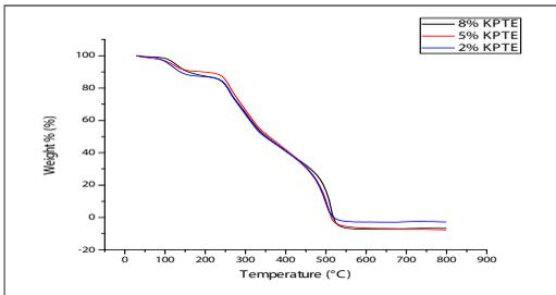
Figure 10: Thermal stability curve of (2, 5 and 8 wt%) kenaf fibres epoxy composites
