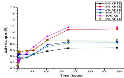
Figure 11: Graph of water uptake of kenaf/PET/epoxy composites
