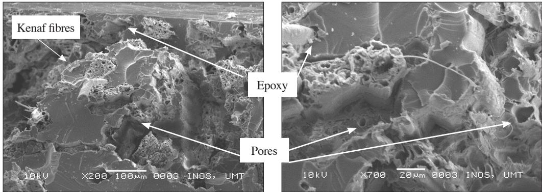
Figure 7: SEM micrograph of the cross section of 10 wt% kenaf/epoxy (KE) composites at a) 200 × magnification and b) 700 × magnification
