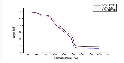
Figure 9: Thermal stability curve of (0 and 10 wt%) kenaf fibres composites and 10 wt% PET composites
