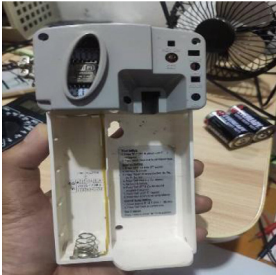
Figure 8: The internal view of iMOS dispenser with the attached X'MOS-circuit board
