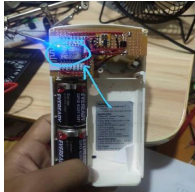
Figure 9: The view of X'MOS-IOT circuit board inside the upper cover
